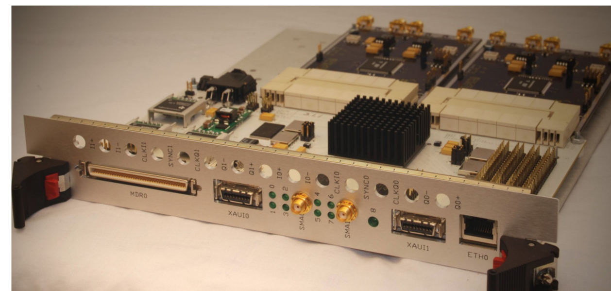
Figure 3. IBOB: The Internet Break-Out Board. The IBOB has two CX4 connectors for high-speed I/O. Two 1GSa/sec ADC boards are attached to the IBOB.
